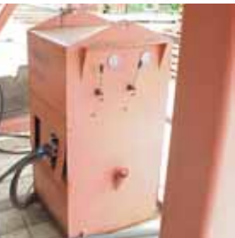
200 bar hydraulic power unit and control console, capable of operating up to 4 lifting brackets, with automatic fail safe flow control
